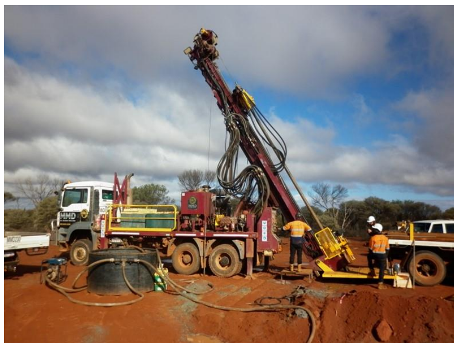
Figure 4 – Stage 10 diamond core rig drilling core tails
